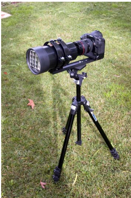
Figure 6: Our sparse light field camera prototype, with 2 positive lenses and an array of 20 negative lenses in front of a conventional camera.
