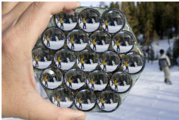
Figure 4: Our optical device consisting of lens-prism pairs.
