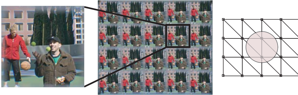
Figure 5: The set of 20 images (middle) is a sparse light field captured with our camera. A close-up of one of the images is shown on the left. The hazy edges are defocused images of the boundaries of the lenses; for the results in this paper, we discard these contaminated pixels. Each vertex on the right represents one camera view. We decompose the camera plane into triangles illustrated on the right. Any novel camera view inside these triangles can be synthesized using tri-view morphing. The circular region represents a possible virtual aperture we want to simulate.
