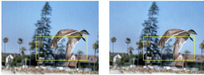
Fig. 7. Stereo images from our mask-based camera. Stereopsis can be achieved with crossed eye observation. Close examination of the marked areas will also reveal horizontal parallax between the pictures.
