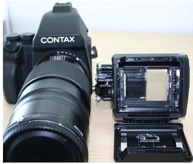
Fig. 5. Our camera with the 3M filter in the film back.
