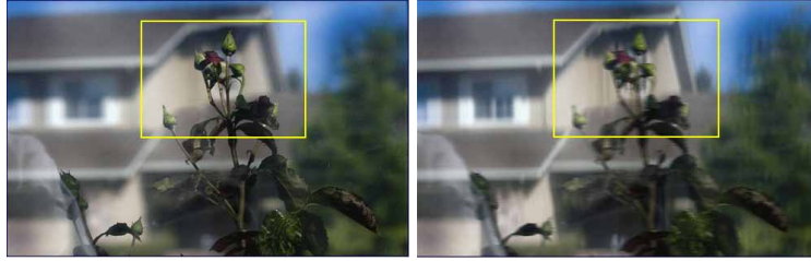
Fig. 8. Refocused images from our mosquito-net-based camera.
