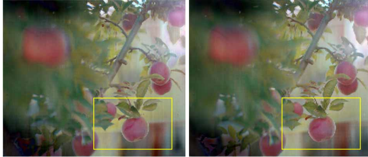
Fig. 9. Stereo images from our lens-based camera. Stereopsis can be achieved with crossed eye observation. Close examination of the marked areas will also reveal horizontal parallax between the pictures.
